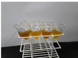
Harle-Tsu raw material extract by SFE with the same pressure and temperature. The CO<sub>2</sub> mass and vegetable mass was variable.
