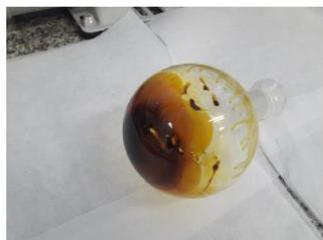
Extracts A, B, C and D were collected and the solvent was removed in rotary evaporator.
